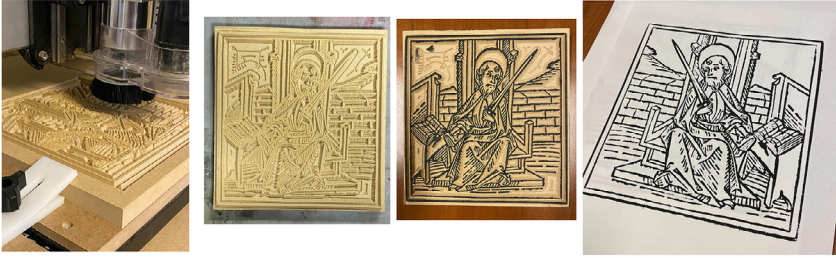
Image 5: The process of making and printing a CNC woodcut
