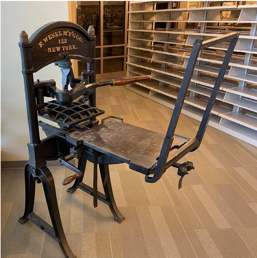
Image 1: Washington style printing press
